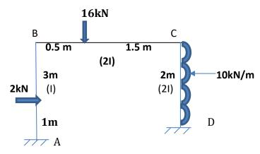
**10** Analysis the portal frame as shown in fig and draw BM diagram.
