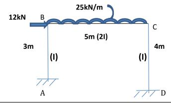
7 Analysis the portal frame as shown in fig and draw BM diagram.
