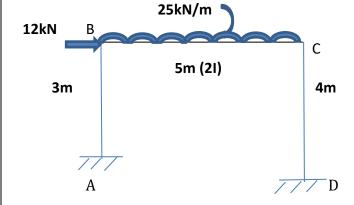
11 Analysis the portal frame (non sway) as shown in fig and draw BM diagram.
